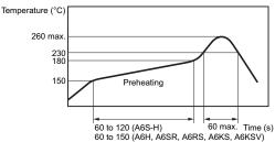
The soldering conditions and the temperature around the Switch may vary with the type of reflow bath. Check the temperature profile and confirm soldering conditions as well as the amount of heat applied to the Switch prior to soldering.
