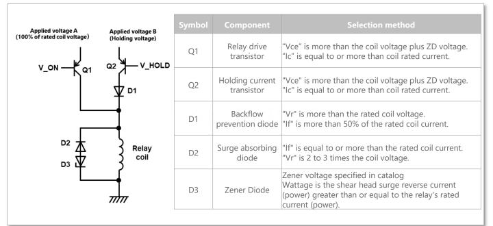
Figure 24: Recommended holding voltage circuit example with switch, and peripheral component selection method
