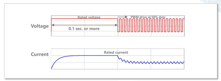
Figure 27: Example of coil voltage and current waveforms in PWM control circuits
