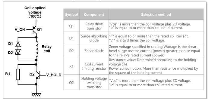
Figure 22: Recommended holding voltage circuit example with switch, and peripheral component selection method
