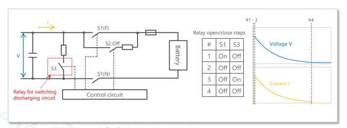
Figure 6: Application example for discharging circuits in ESS
