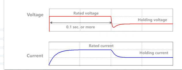
Figure 21: Example of coil voltage and current waveforms in CR circuit
