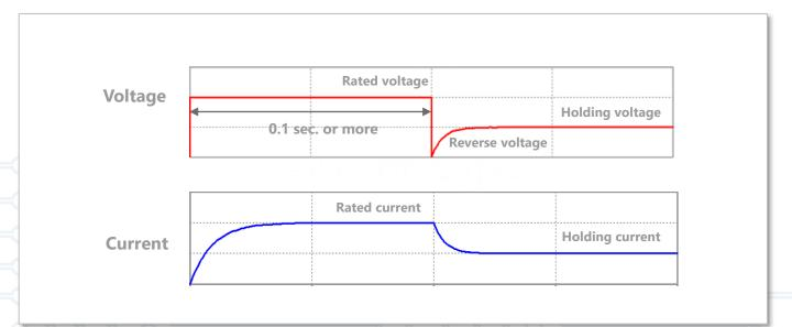
Figure 23: Example of coil voltage and current waveforms in holding circuit with switch
