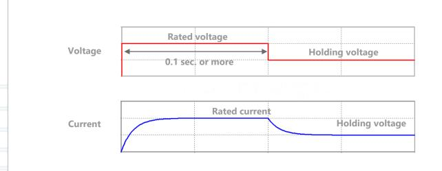
Figure 25: Example of coil voltage and current waveforms in holding circuit with switch
