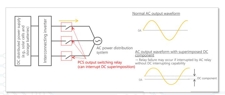
Figure 7: Example of use of DC superimposition interruption of AC circuit in PCS
