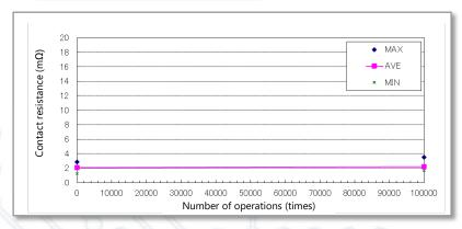
The contact resistance after 30 seconds at 6 VDC, 20 A measured using the voltage drop method. (Ambient temperature 23°C)
