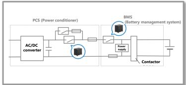
Figure 1: Example of Power conditioner and Battery Unit relay application
