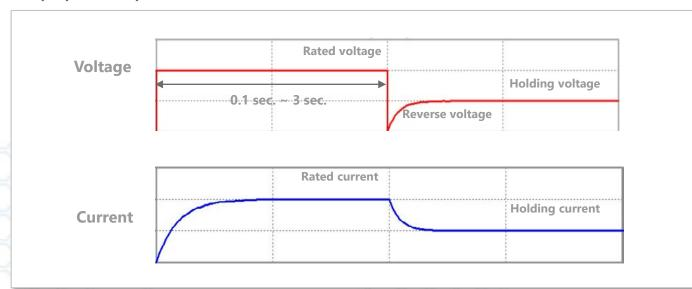
Figure 19: Example of coil voltage and current waveforms in holding circuit with switch
