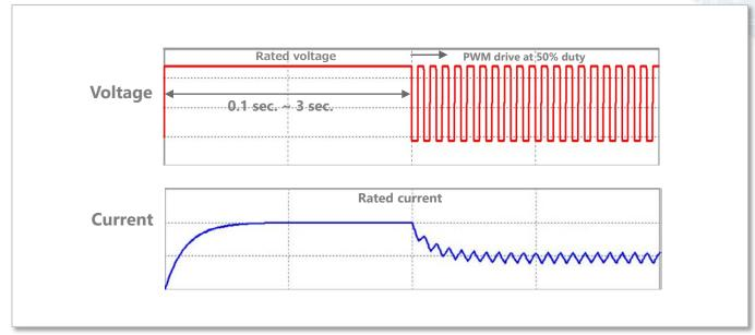
Figure 23: Example of coil voltage and current waveforms in PWM control circuits
