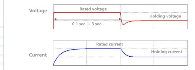
Figure 17: Example of coil voltage and current waveforms in CR circuit
