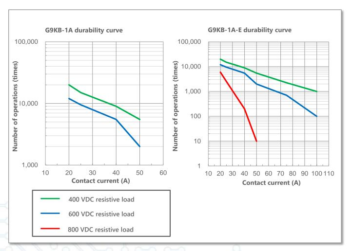
Figure 13: G9KB series durability curve
