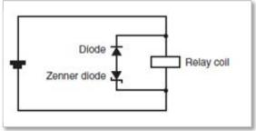
Figure 14: Diode connection
