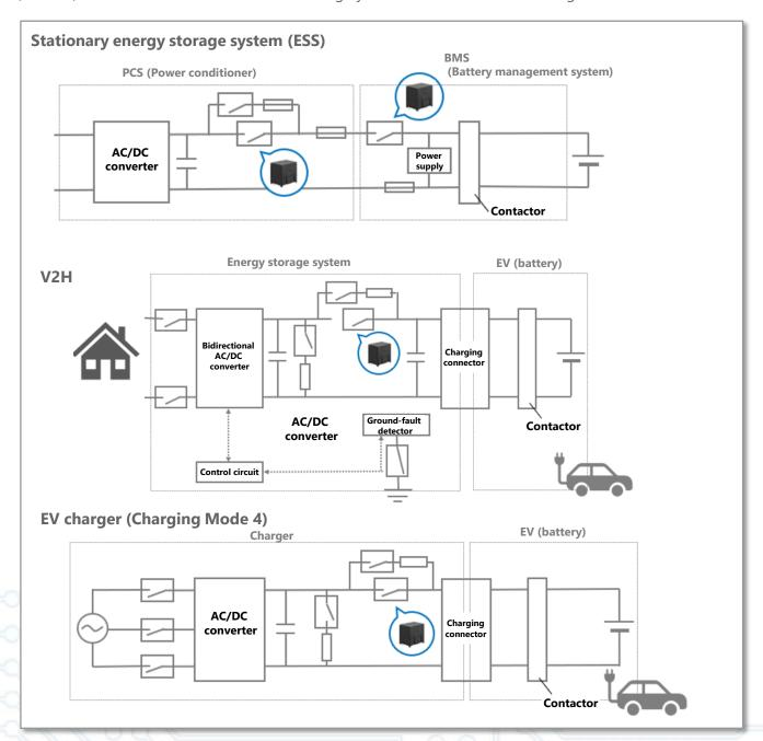
Figure 4: Example of use with ESS, V2H, and EV chargers
