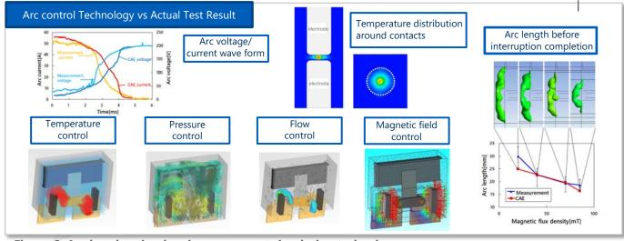
Figure 6: Analyzed optimal arcing movement simulation technology
