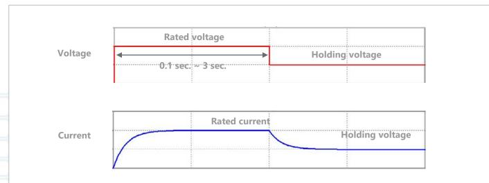
Figure 21: Example of coil voltage and current waveforms in holding circuit with switch
