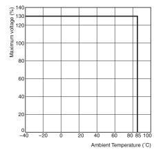
Note. Maximum voltage of set pulse and reset pulse at duty factor 10% (Maximum pulse width: 1min).
