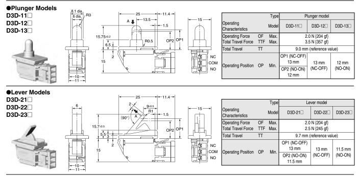
Note 1. Unless otherwise specified, a tolerance of  $\pm 0.4$  mm applies to all dimensions. Note 2. The operating characteristics are for operation in the A direction ( $\clubsuit$ ).
