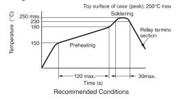
Note: Do not dip the Relay into the solder bath. Doing so may cause malfunction due to plastic deformation.
