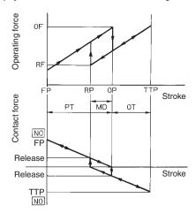
Make sure that the operating body is set so that the actuator should return to the free position when the operating body has moved if a switch is used to form a normally closed (NC) circuit. If a switch is used to form a normally open (NO) circuit, the operating body must move the switch actuator to the distance of 70% to 100% of the rated overtravel (OT) of the switch.
