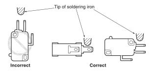
When soldering automatically, adjust the amount of solder so that flux does not float onto the top of PCB. If flux enters the switch, it can cause contact failure.
