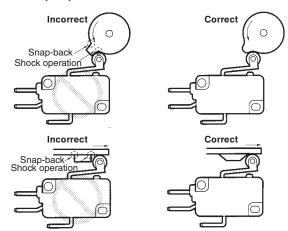
Make sure that no improper force is applied to the actuator, otherwise the actuator may incur local abrasion. As a result, the actuator may become damaged or its durability may be deteriorated.
