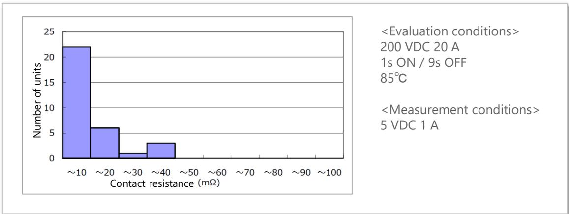
Figure 15: G5PZ-X initial contact resistance (for one contact)
