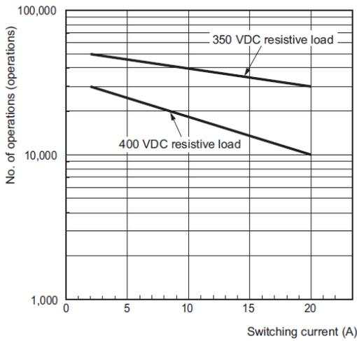
**Figure 17: Electrical durability**
