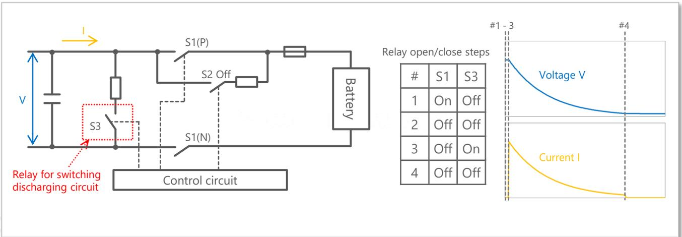
Figure 6: Application example for discharging circuits in ESS
