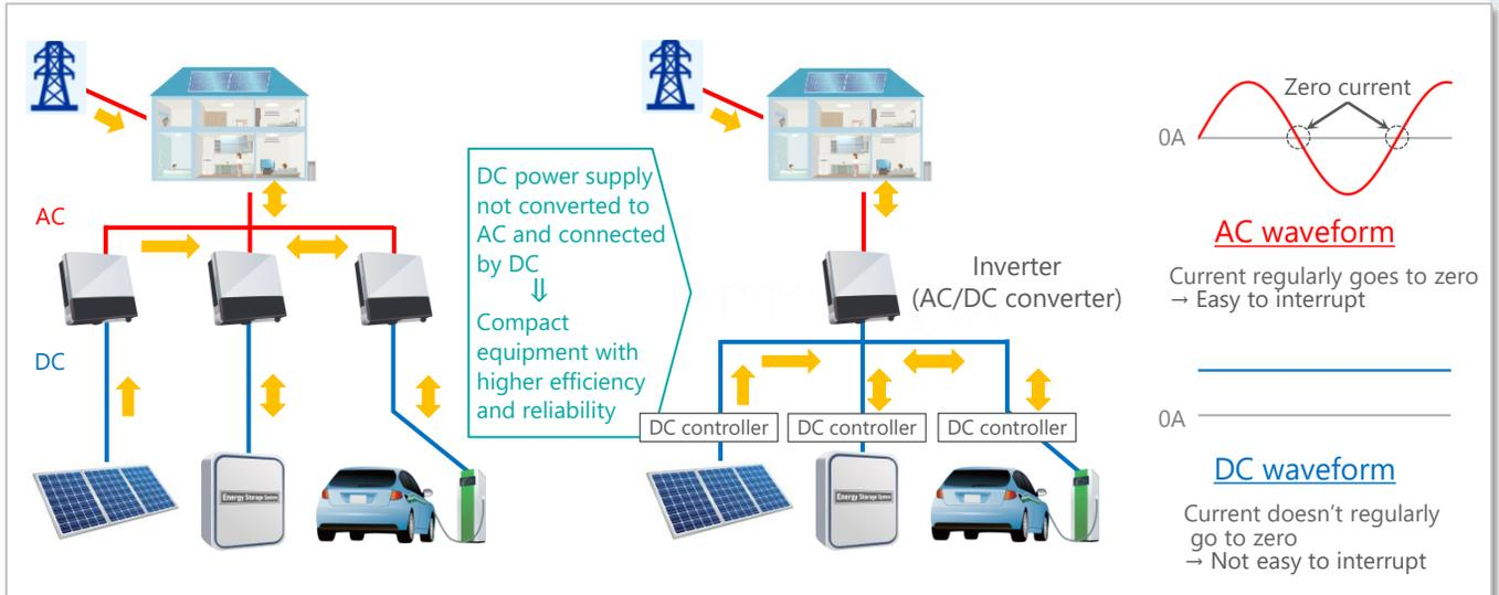
**Figure 3: AC and DC interconnections of various DC distributed power supplies (DC link)**
