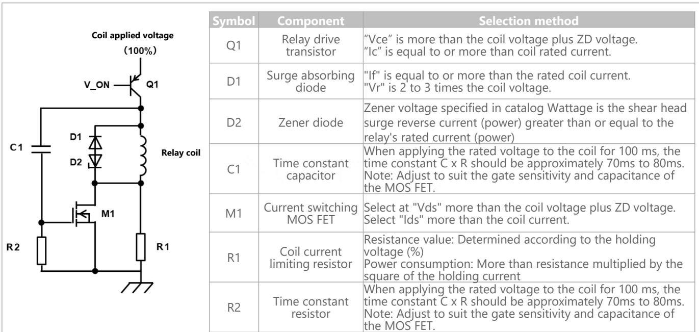
Figure 20: Recommended holding voltage CR circuit example and peripheral component selection method
