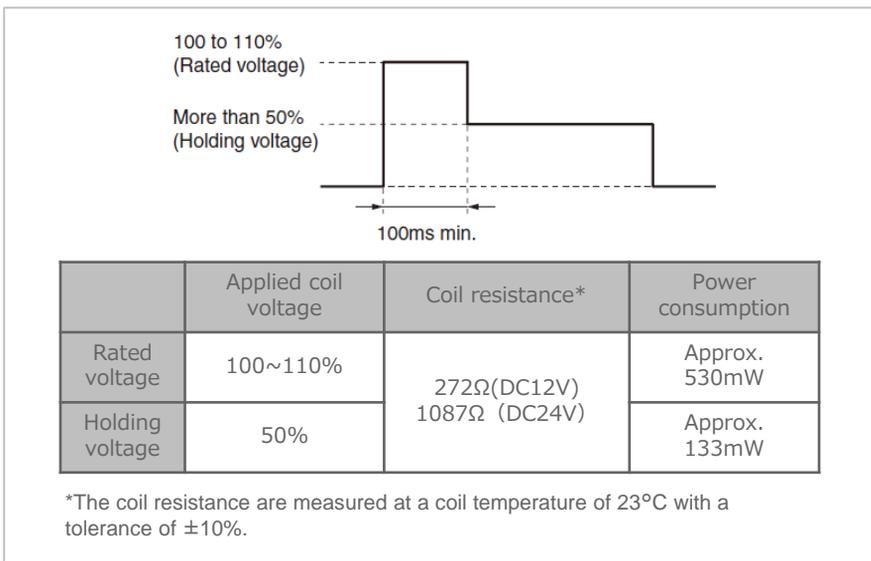
Figure 10: Coil voltage reduction after relay operation (holding voltage)
