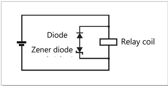
Figure 18: Diode / Zener diode connection
