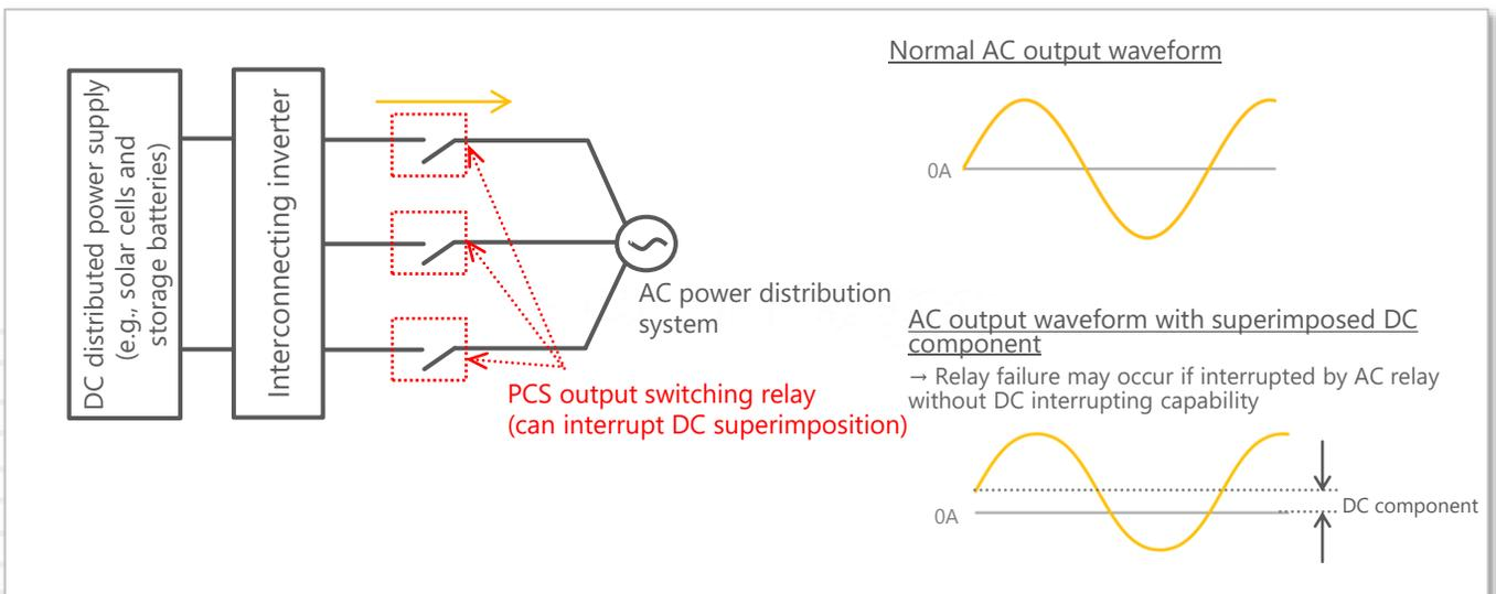
Figure 7: Example of use of DC superimposition interruption of AC circuit in PCS
