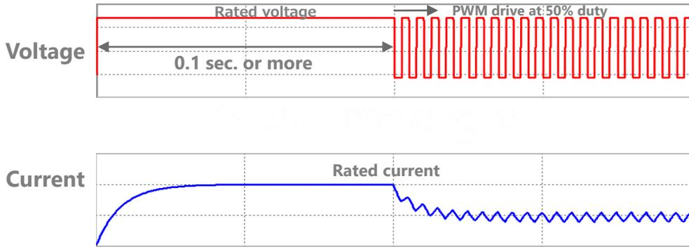
Figure 27: Example of coil voltage and current waveforms in PWM control circuits
