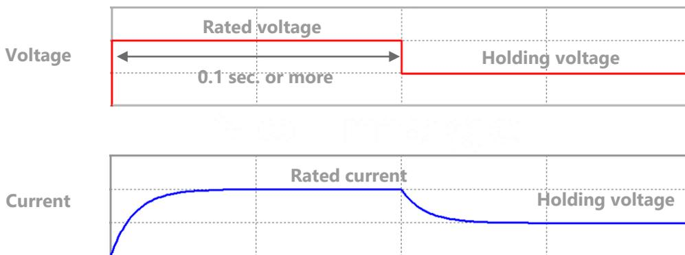
Figure 25: Example of coil voltage and current waveforms in holding circuit with switch
