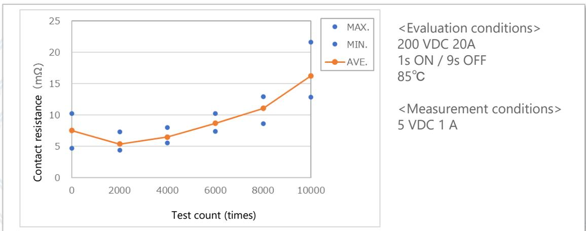
Figure 16: G5PZ-X contact resistance after electrical durability testing
