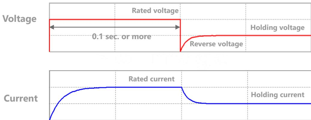
Figure 23: Example of coil voltage and current waveforms in holding circuit with switch
