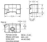
Note: If you use a Dust Cover with a holding ring, secure the holding ring at part A.
