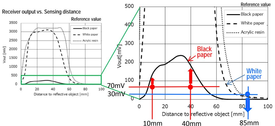
When designing your actual application, the sensing distance should be properly determined by first referencing the graph of "Receiver output vs. Sensing distance." In the case that the sensing object position does not fluctuate, the sensing distance is recommended to be set at the peak of the graph's curve.
