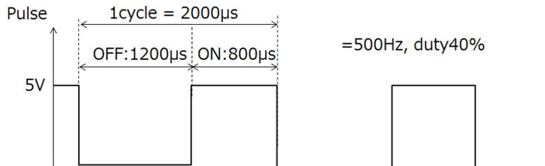
Notes: \*On time (Pulse width): When pulsing the LED, the output becomes stable within 400 micro sec., max. Therefore 800 (>> 400) micro sec. of on time is recommended, to ensure proper operation.
