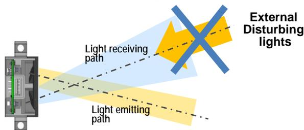
3. In the case of attaching a transparent cover on the sensor for water/dust prevention purpose, the plate must be closely attached to the sensing surface of the device. Depending on the thickness of the cover plate, the reflected light at the inside surface of the plate will reach the sensor receiver. Therefore, proper evaluation should be performed, especially for the super compact type which has a short sensing distance and a fixed threshold level.
