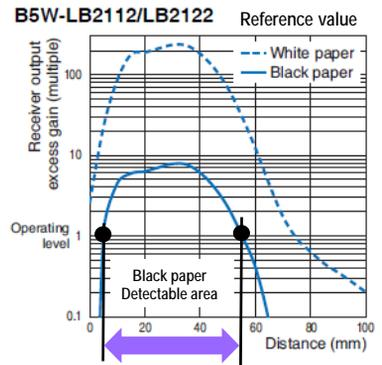
Please see “Operating range characteristics” (reference value) below. The curve in this graph shows operating points (turn OFF to ON with Light –ON type) when an object to be sensed travels in the arrow’s direction for each sensing distance.
