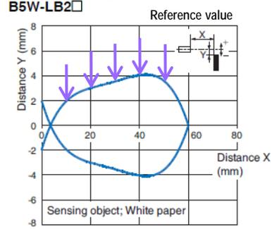
In the case of detecting moving objects, a reflective type sensor is generally mounted vertically to the surface on which the light emitting axis and the light receiving axis are crossing (equal to “Left and right” direction).
