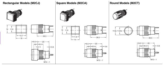
Note: Unless specified, there is a tolerance of  $\pm 0.4$  mm for dimensions.
