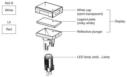
Ordering: With colored-illumination models, order the Display, Lamp, and Socket Unit as shown in the following table.
