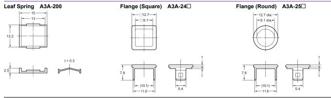
Note: Unless otherwise specified, a tolerance of ±0.4 mm applies to all dimensions.
