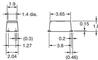
Unless otherwise specified, the dimensional tolerance is  $\pm 0.1$  mm.
