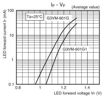
Trigger LED forward current vs.
