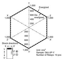
Test Conditions: Shock is applied in ±X, ±Y, and ±Z directions three times each with and without energizing the Relays to check
