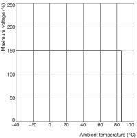
Note: "Maximum voltage" is the maximum voltage that can be applied to the Relay coil. Shock Malfunction
