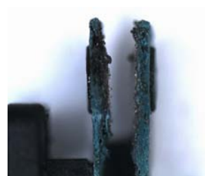
Corrosion at the contact
