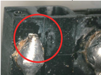
Trace that liquid adhered.
