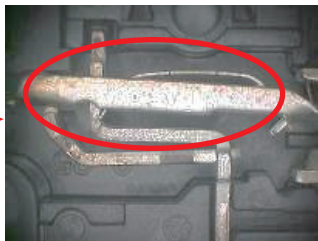
Trace of liquid penetration
