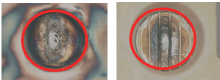
Contact is sulfurized
