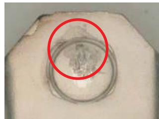
The corroded substances are generated.
