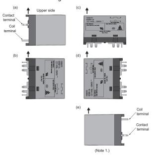
Note 1. The operating voltage differs from the applied coil voltage for contact terminals mounted in the downward direction (e). Please refer to ●Coil on page 2 and ●Coil Voltage Reduction (Holding Voltage) during and after Relay Operation.
