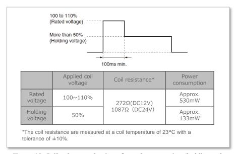
Figure 10: Coil voltage reduction after relay operation (holding voltage)
