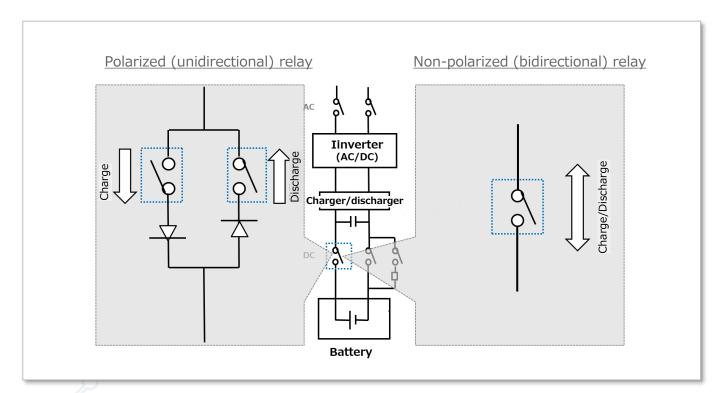
Figure 9: Bidirectional switching
