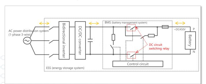
Figure 4: Example of use of DC circuit switching in ESS
