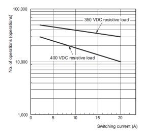
Figure 17: Electrical durability
