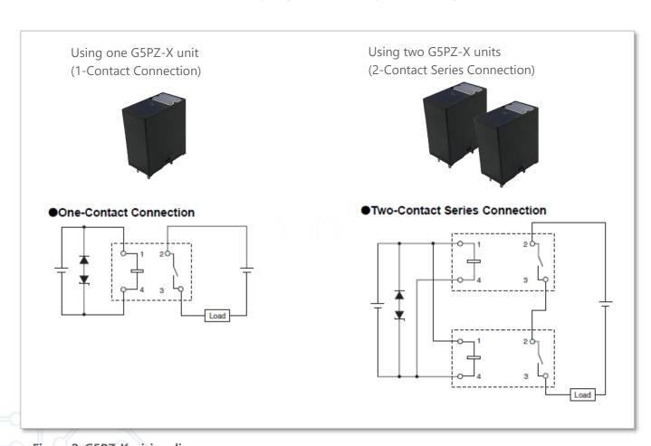
Figure 8: G5PZ-X wiring diagram
