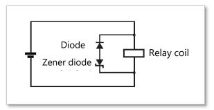
Figure 18: Diode / Zener diode connection
