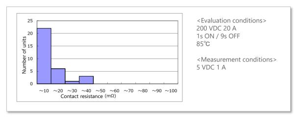
Figure 15: G5PZ-X initial contact resistance (for one contact)
