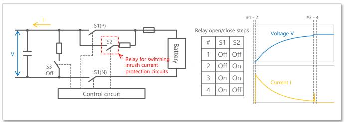
Figure 5: Application example for inrush current prevention circuit (precharge circuit) in ESS
