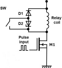
\* Due to the Zener diode, the PWM circuit may not operate as expected.
