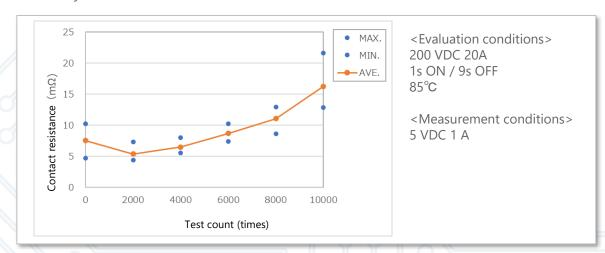
Figure 16: G5PZ-X contact resistance after electrical durability testing
