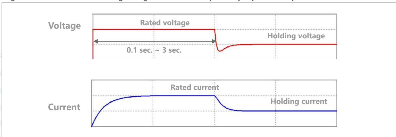
Figure 17: Example of coil voltage and current waveforms in CR circuit
