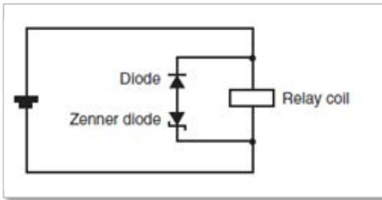
Figure 14: Diode connection
