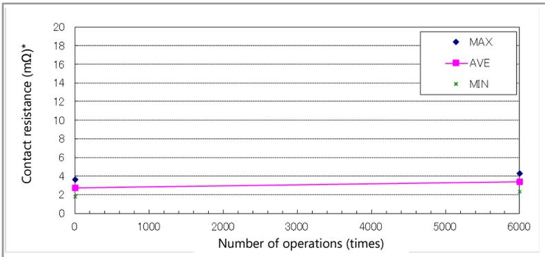
The contact resistance after 30 seconds at 6 VDC, 20 A measured using the voltage drop method. (Ambient temperature 23°C)
