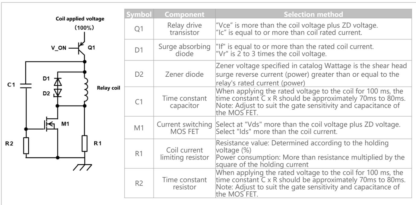
Figure 16: Recommended holding voltage CR circuit example and peripheral component selection method
