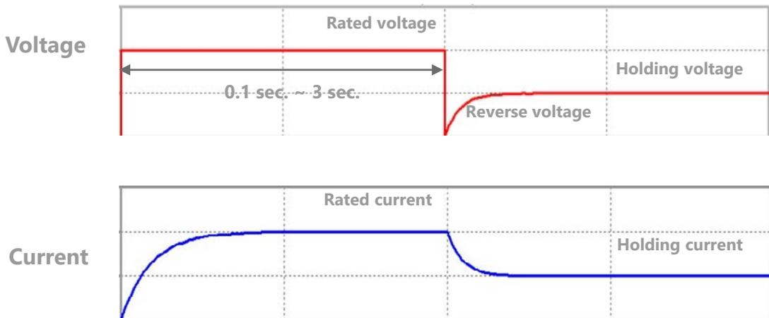
Figure 19: Example of coil voltage and current waveforms in holding circuit with switch
