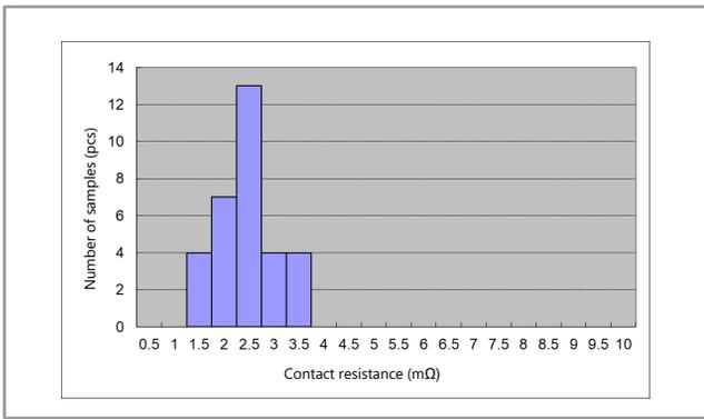
Figure 9: G9KB series initial contact resistance (measured value)
