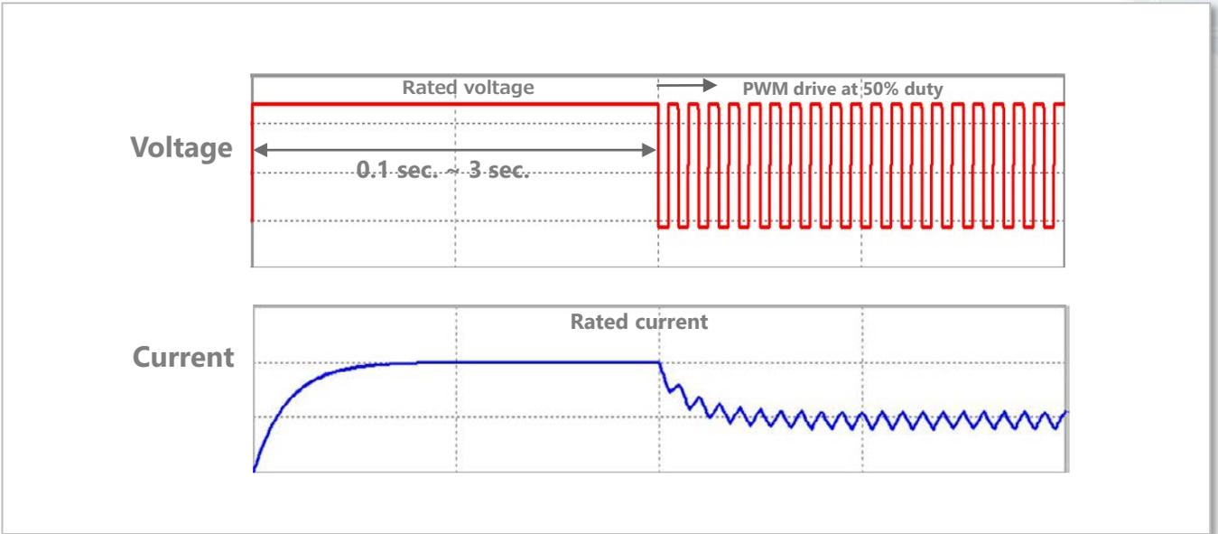
Figure 23: Example of coil voltage and current waveforms in PWM control circuits
