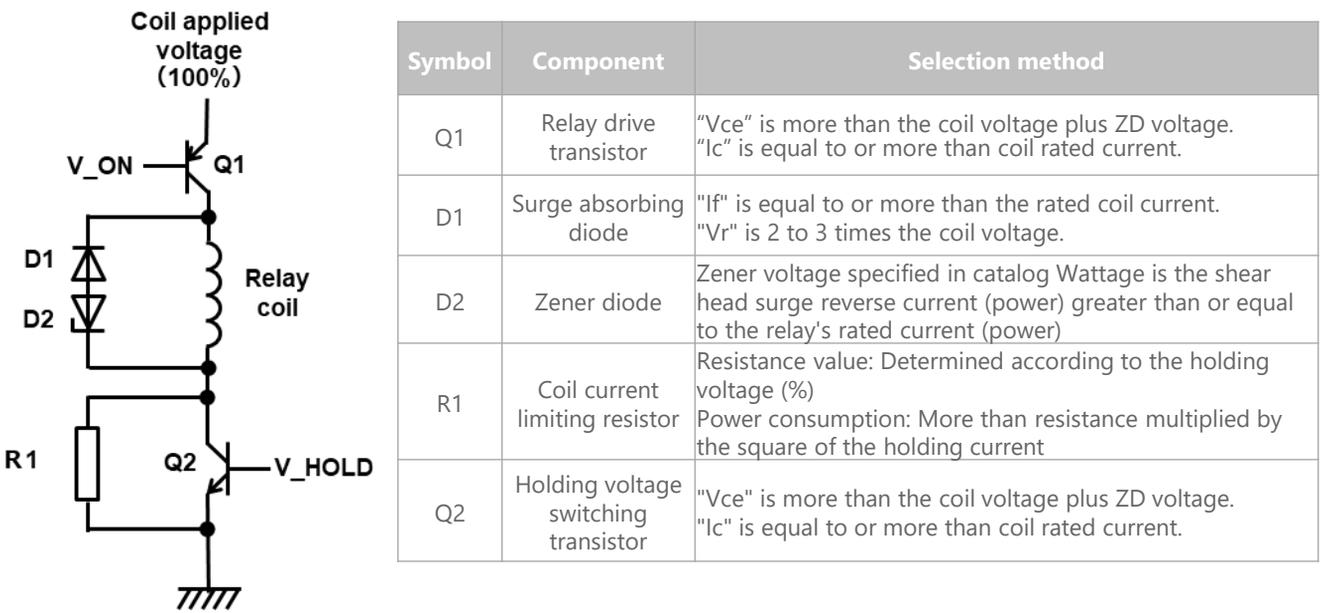
Figure 18: Recommended holding voltage circuit example with switch, and peripheral component selection method
