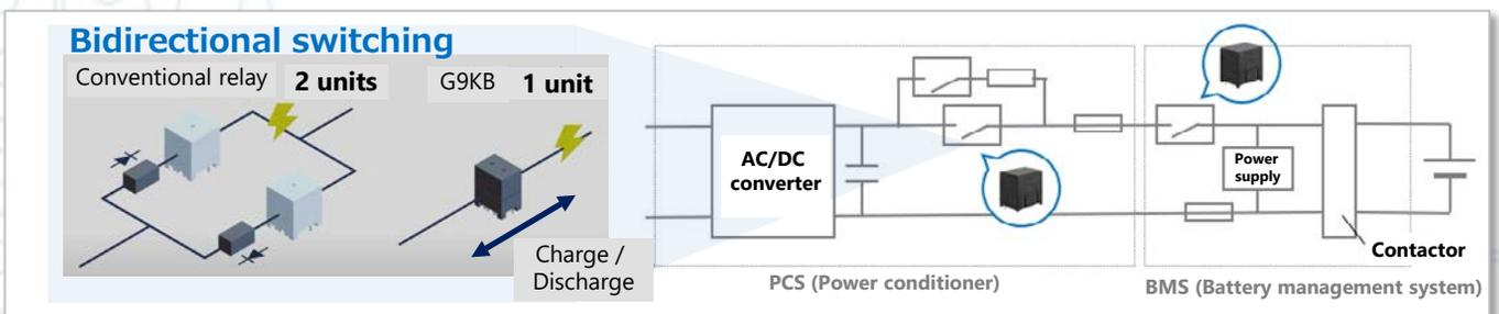
Figure 7: Bidirectional switching applications in energy storage system
