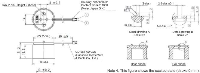
\* The dimensional tolerance must be ±0.5 unless otherwise specified.
