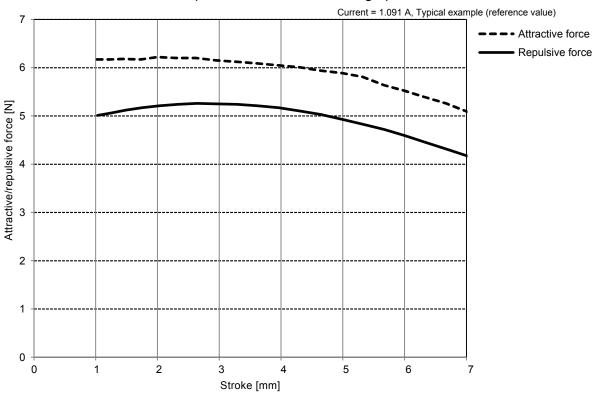
Note 7: Measured by placing this product vertically, fixing the bobbin, and driving the case.
